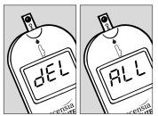
**3** The Display begins flashing **dEL** and **ALL** every second for 5 times, and then the Display goes blank. Do not pull the Check Strip out of the Meter until the Display goes blank, or the stored test results will not be deleted.
